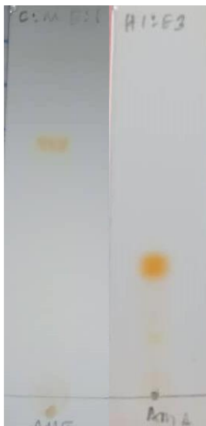
Plate II: TLC Chromatogram of the isolated compound using chloroform: Methanol 4:1 and Hexane: ethylacetate 1:3
