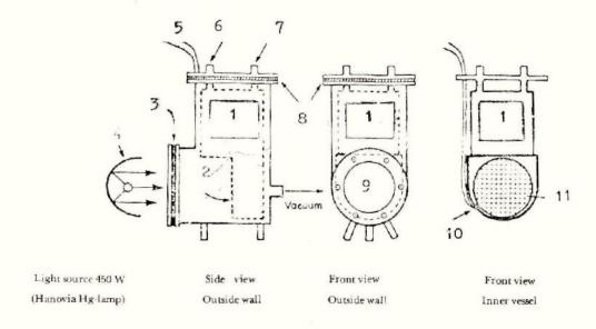
Fig. 6: Apparatus for the irradiation of solid substances (acc. to Scheffer and Dzakpasu, 1978).
